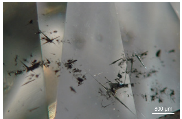
Figure 13: Many black needle-like inclusions are present in the Banjarmasin diamond, and they are commonly oriented in specific (mainly octahedral) directions. Photomicrograph by J. C. Zwaan.
